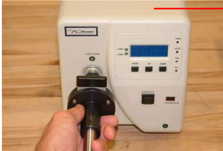
Figure 16 Lamp output test adapter connected to Omnicure S2000.
