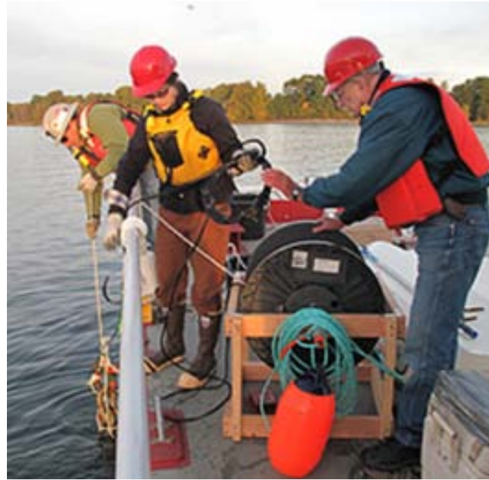
Underwater blast on the Columbia River. Aimone-Martin Associates did all the underwater pressure measurements.
