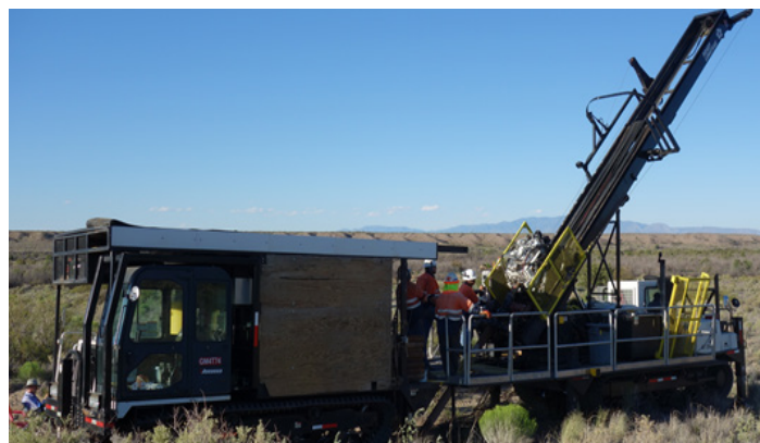
Fig. 3 Coring across the Loma Blanca fault: collection of fault zone and host sediment samples
