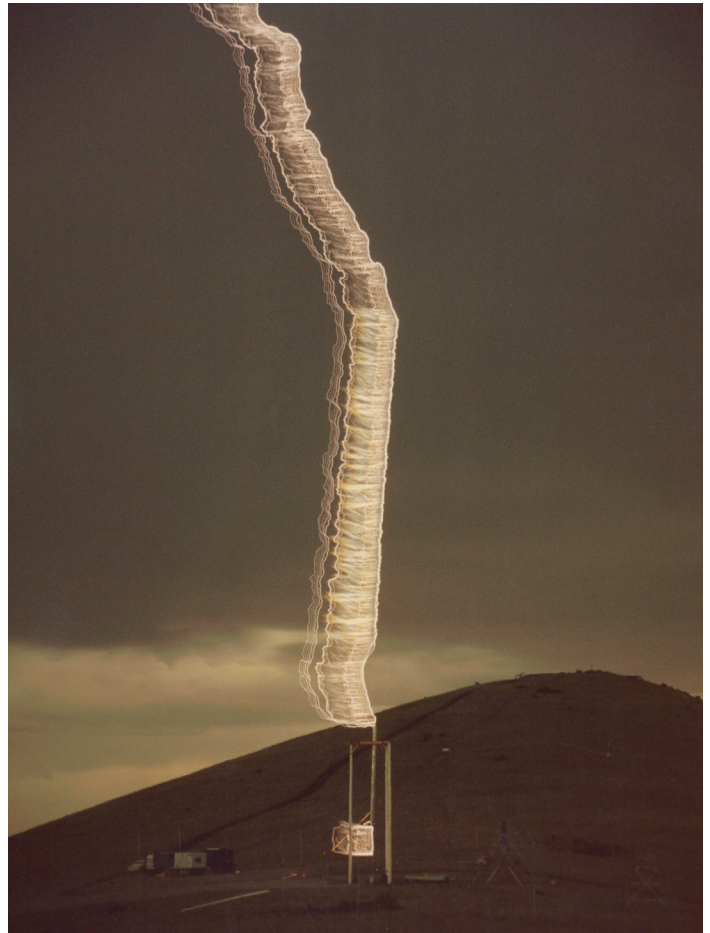
Dramatic photo of an early experiment in lightning triggering. A wire-trailing rocket caused a lightning flash and the current traversed (and vaporized) the wire. The sheetlike appearance of the lightning is caused by "streamers" and strong winds during multiple strokes.
