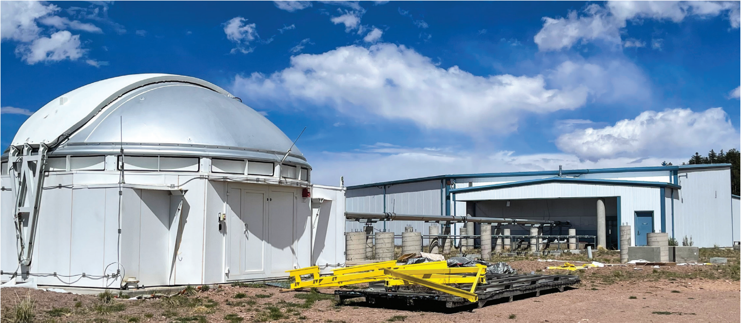
The first MROI telescope located on the array outside the Beam Combining Facility. The yellow frame on the ground is used to lift the telescope and enclosure together as a unit and move them to a new station on the array. The second telescope will be located adjacent to the first telescope later this month and used this fall to make the first MROI measurements of interference fringes on stars.
