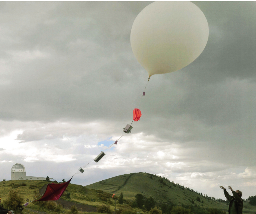
A balloon train begins its ascent into a thunderstorm from the Langmuir Lab balloon hangar. Multiple instruments along the string measure X-rays, electric fields and provide a location to allow instrument recovery.
